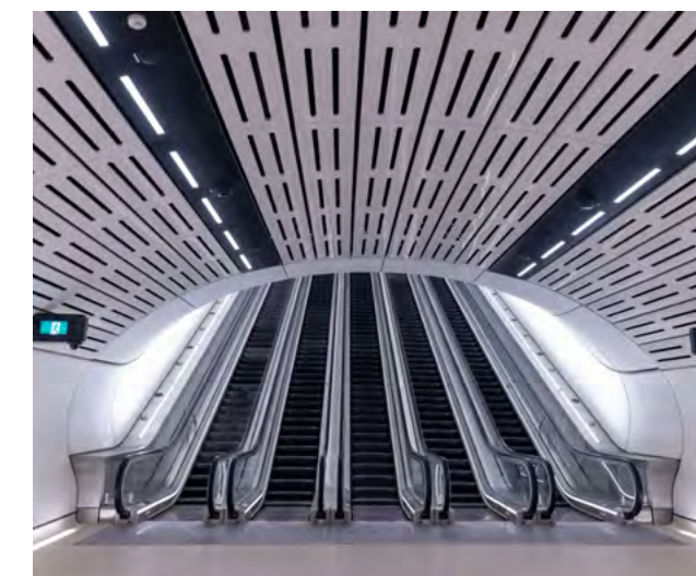
Image: The internal acoustic insulation at Victoria Cross station is made from up to 80 per cent recycled PET plastic packaging such as drinking water bottles.
